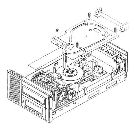
Figure 8-9. Threader Assembly
